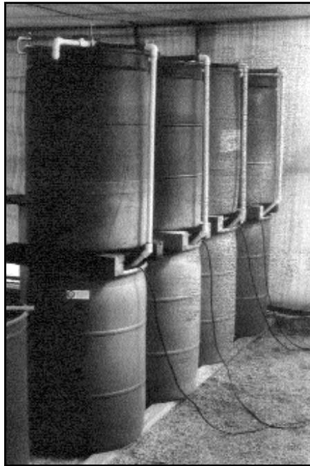
*The Cabrillo Organic Tea Project double-barrel active tea extractor units #1-4, set up in the greenhouse. The four passive extractors (#5-8) were single-barrel units (not shown).*
