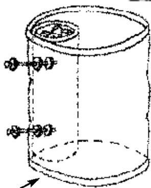
**Fig. 8.** Packed column filled with 4 inch PVC pieces, bolted inside of top barrel; a gravity-fed aeration system.
