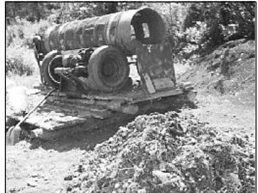
A drum type screening system.
