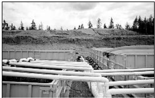
A prototype in-vessel composting operation. This method involves considerable equipment and investment.
